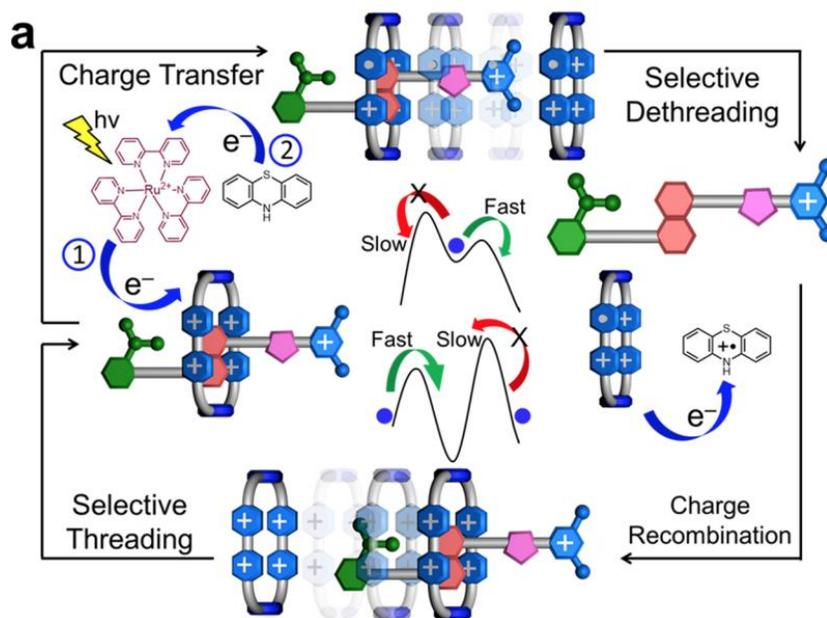
Figure 12 (a): mechanism for the photochemically induced redox-driven [2]pseudorotaxane based on macrocycle  $\text{CBPQT}^{4+}$  and axle  $\text{D1}^+$ . Adapted from Stoddart et al [21]
