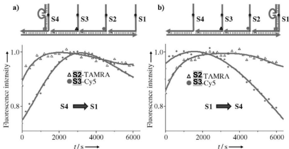
Figure 7: Graphical FRET assay representation of the progressive movement. Donor fluorophore FAM labeled walker moves on anchorage sites 2 and 3 both labeled with a suitable acceptor, TAMRA and Cy5 respectively Adapted from You et al [16].
