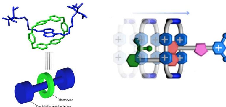
Figure 10 Left: Dumbbell shaped rotaxane consisting of macrocyclic ring and asymmetrical axle. Right: Pseudorotaxane, rotaxane type structure allowing for slippage (threading/dethreading) at the end of the less bulk end group; Adapted from Stoddart et al [21]
