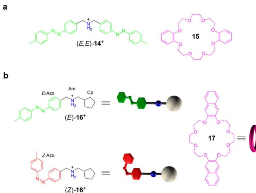
Figure 13 (a): Structural conformation of axle **14<sup>+</sup>** in its E,E configuration along with dibenzo[24]crown-8 macrocyclic ring. (b) Isomerization of synthesized axle **16<sup>+</sup>** capable of slipping into the macrocyclic ring **15** at a faster rate than that over the Z-Azobenzene moiety of **Z-16<sup>+</sup>**. Adapted from Credi et al [12].
