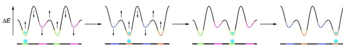
Figure 3: Operation of an energy ratchet with alternating minima and maxima that are modulated to move the black particle directionally. Adapted from Credi et al [12]
