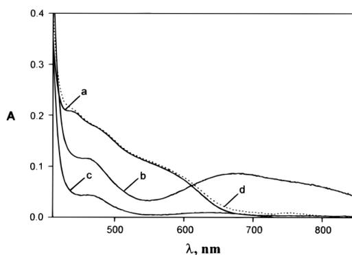
Figure 2 (a) spectral data prior to light excitation, (b) data corresponding to absorption of Cu<sup>I</sup>N<sub>4</sub> in acetonitrile for 20 minutes, (c) after 24 hours in the dark, (d) 30 min post addition of ascorbic acid. Adapted from Sauvage et al [9]
