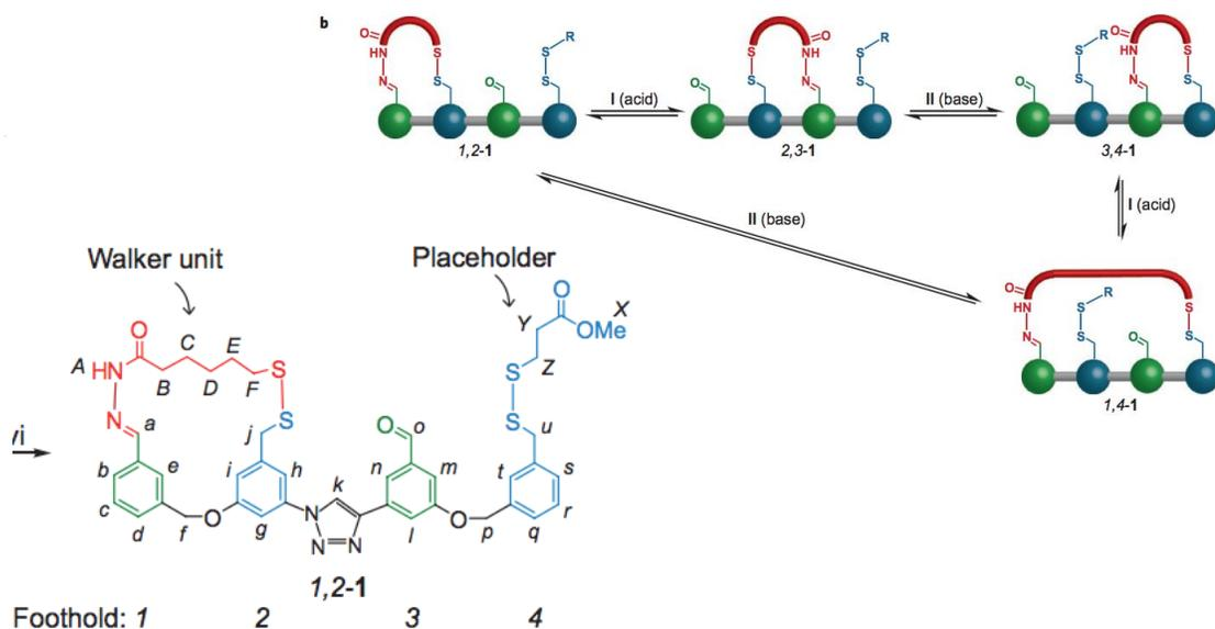
Figure 8a: molecular walker **1,2-1** (numbering designates binding region on track of the walker unit) 8b: operating mechanism based on selectively labile “feet” between the walker (red) and the track. The sequence shows the reversible movement of the walker from left to right under acidic and basic conditions, respectively, Adapted from Leigh et al [19].
