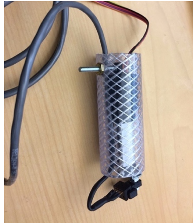
Figure 9. In the image above, we are able to see how the casing in the tonometer helps hold everything together and in place. This is key in order to ensure no loose ends come out and that our tonometer stays functioning.
