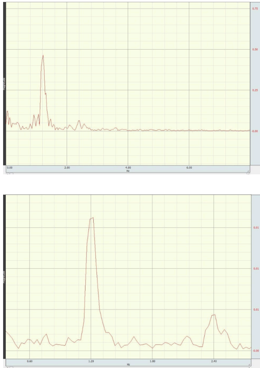
Figure 18. (Top) PPG FFT with a peak at \sim 1.2 Hz (72 BPM). (Bottom) Tonometer FFT with a peak at \sim 1.2 Hz (72 BPM)
