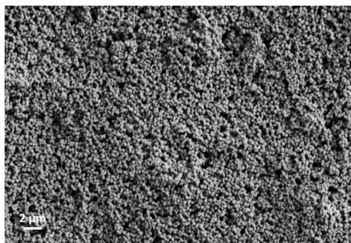
Figure 2.3. SEM image of \text{TiO}_2\text{-(H)} material. The image shows that \text{TiO}_2\text{-(H)} particles have uniform sizes.
