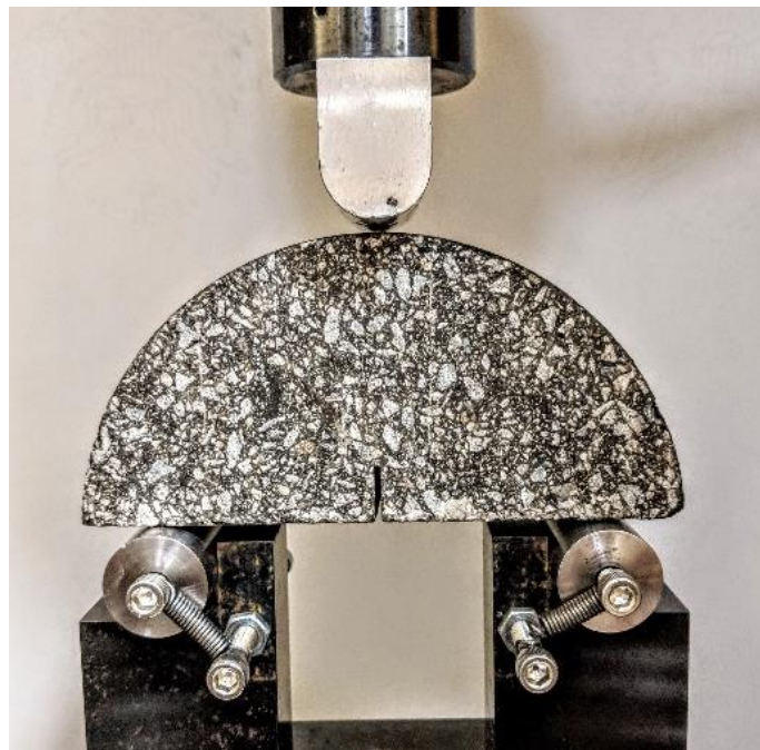
Figure 6: The SCB sample above has been notched to initiate the cracking.
