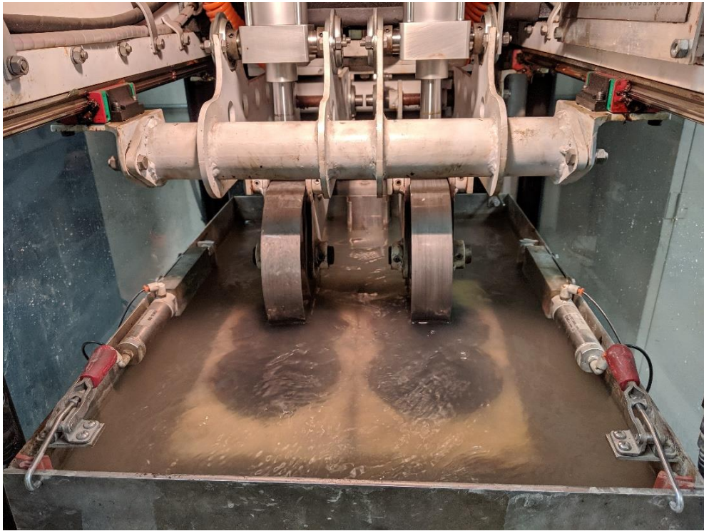
Figure 1: The HWTT is used to measure rutting and moisture susceptibility.
