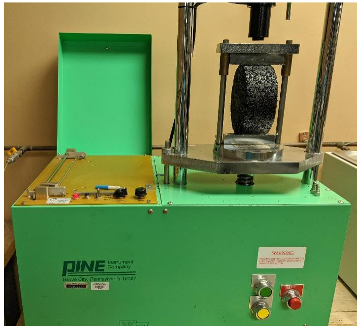
Figure 5: A Pine Instruments compression machine traditionally used for Marshall test specimens at Rutgers University. It has been adapted for IDEAL-CT testing.
