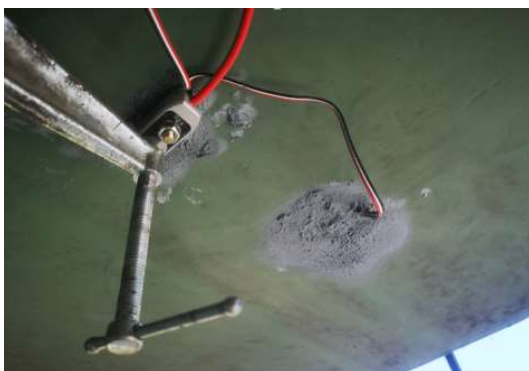
Short-Term Accelerometer Sensor and Deflection Tape
