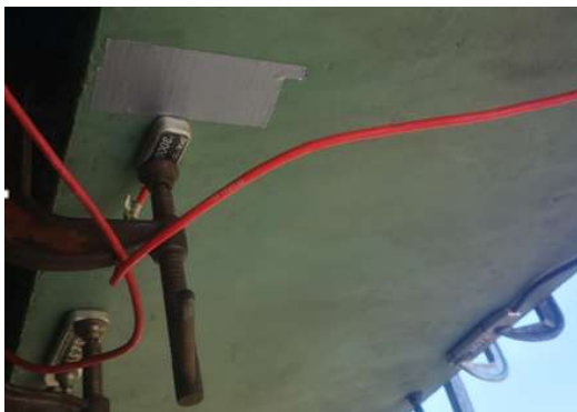
Short-Term Accelerometer Sensor and Deflection Tape
