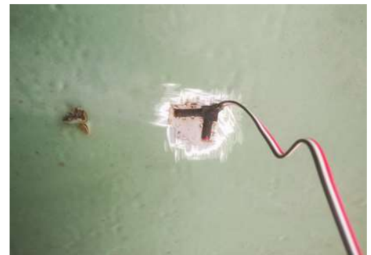
Long-Term Strain Gage (Poisson Gage)
