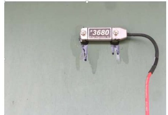
Short-Term Strain Sensor at The Middle Section
