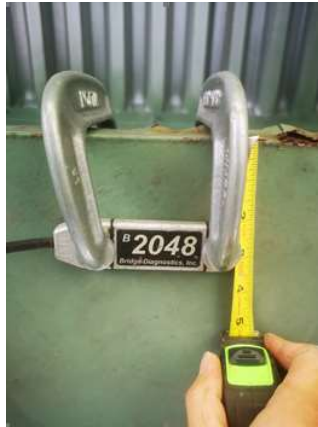
Short-Term Strain Sensor at The Bottom Flange
