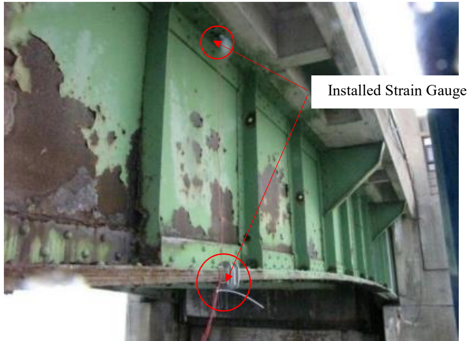
Figure 4.15 - Strain Gauge Placement on top and bottom flange of Fascia Girder
