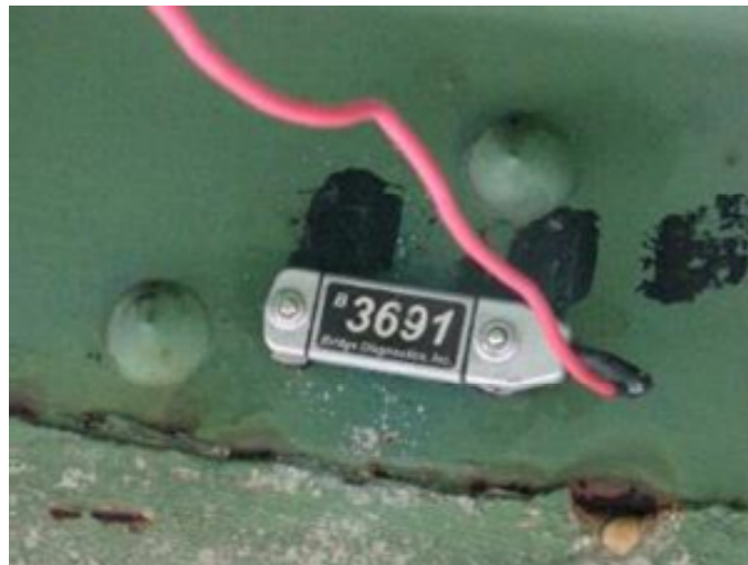
Figure 4.11 - Strain Transducer attached to the top flange of the Fascia Girder
