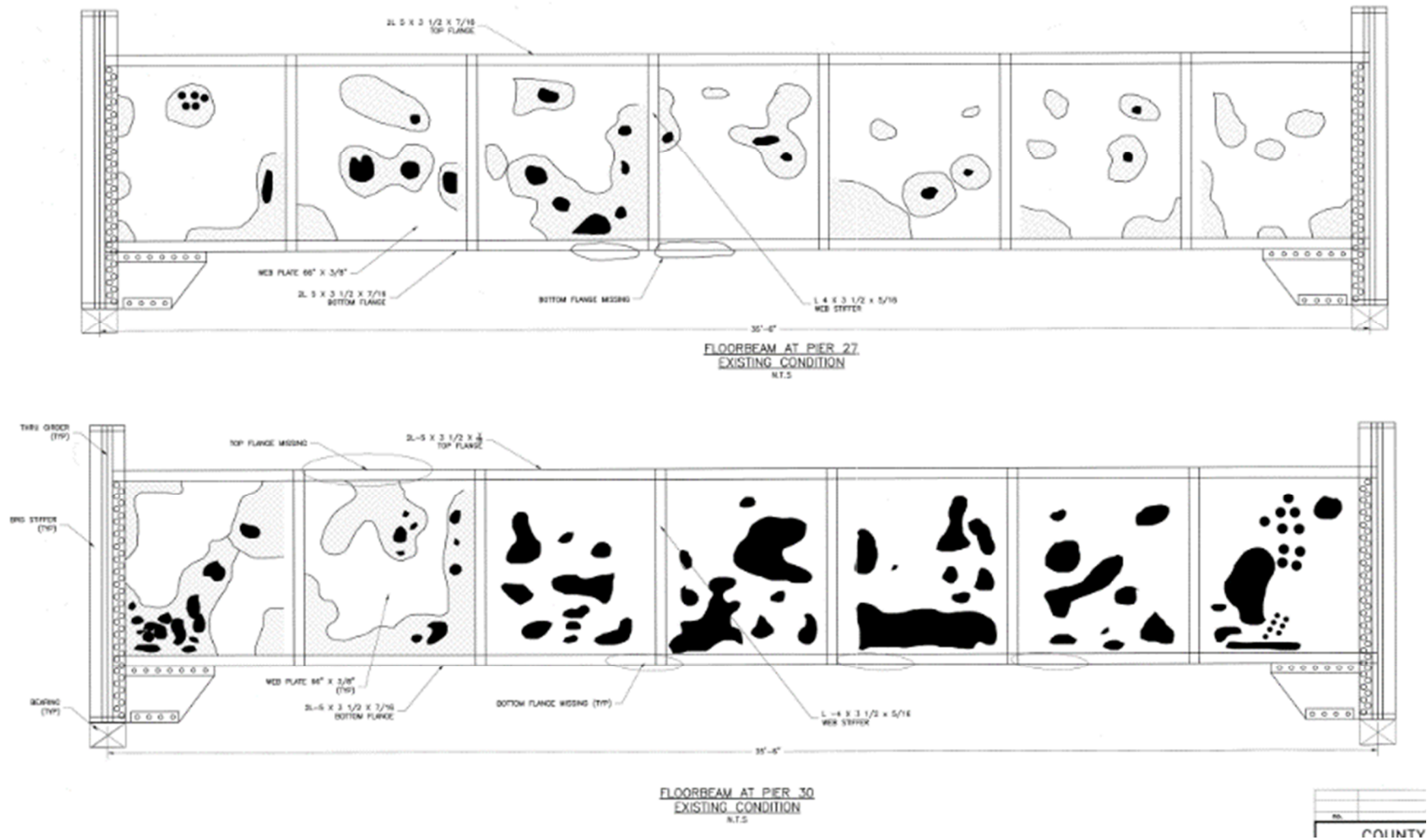
Figure D.8 - Floor Beam Deterioration, Elevation View (2014 Repair Plans)
