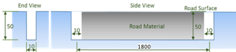
Figure 4.25 - WIM Installation Step 3 WIM Loop Slot
