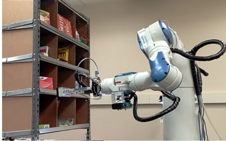
Figure 7.1: A Motoman SDA10F robot carrying the UniGripper tool and an Amazon-Kiva Pod stocked with objects.
