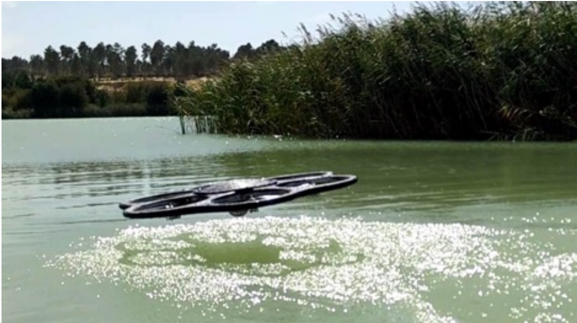
Figure 1.14: Waterproof unmanned aerial vehicle demonstrating aerial flight over water surface. [22]
