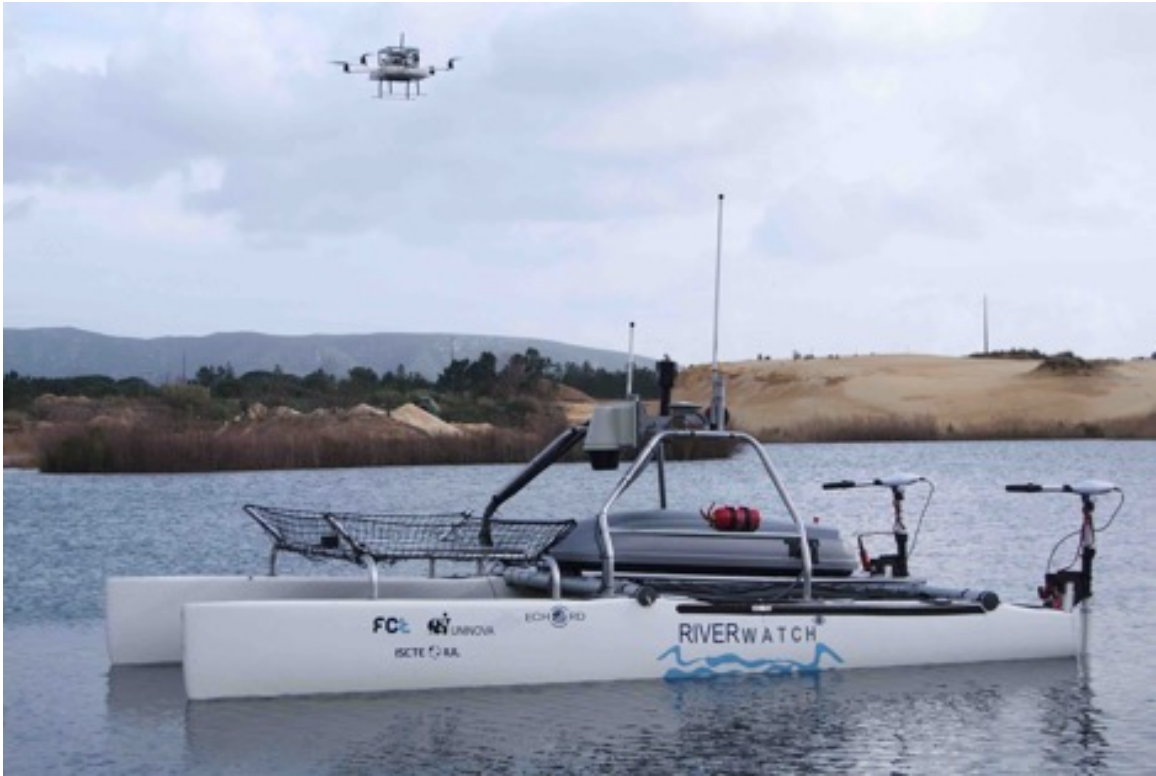
Figure 1.13: Example of a marsupial robotic team composed of an unmanned surface vehicle (USV) and an unmanned aerial vehicle (UAV). [20]
