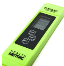
Figure 22: Handheld HEALTH METRIC® EC meter.
