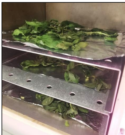
Figure 59: Basil plants being dried in the vacuum oven at 40 °C on day 21 for Treatment 1
