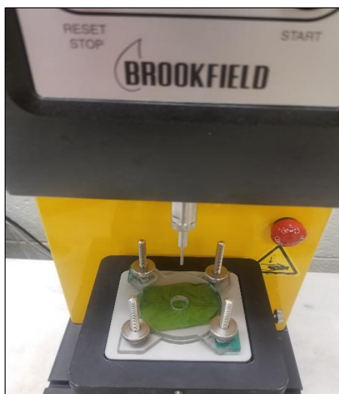
Figure 25: Brookfield CT-3 texture analyzer with a 2 mm diameter probe, modified base plate, and basil leaf held between the circular plastic plates.
