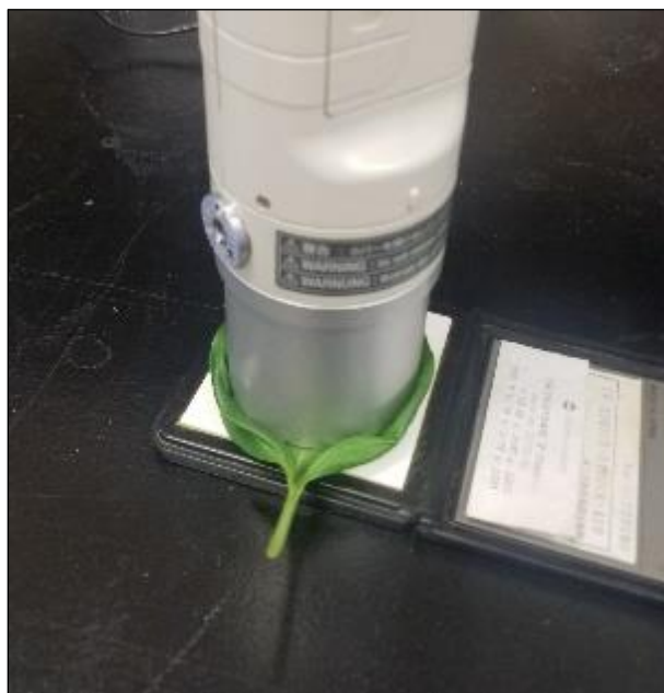
Figure 40: Basil leaf placed on an opaque white plate and its color being measured using Konica Minolta CR-410 colorimeter.
