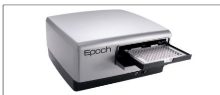
Figure 27: BioTek™ Epoch™ spectrophotometer with a 96 well microplate.
