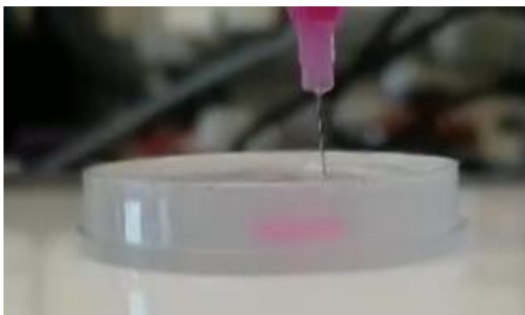
Figure 9. Printed material is supported above the bottom of the slurry container.
