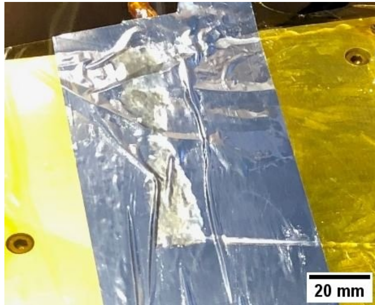
Figure 13. Extrusion of dog-bone model with insufficient curing (carbon fiber and G/Flex mixture)
