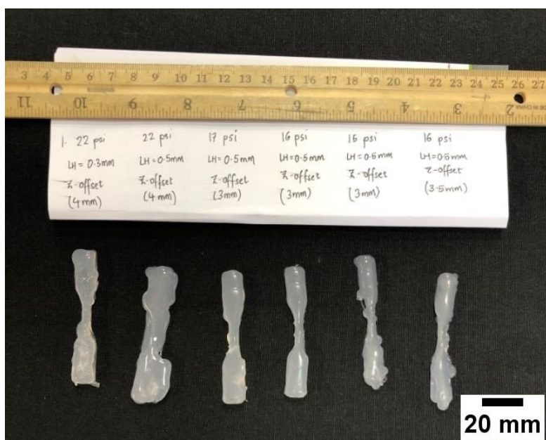
Figure 16. Pure Ecoflex dog-bone-shaped samples (iterative testing by varying layer height, offset height, extrusion pressure)
