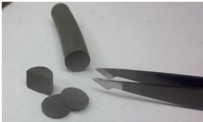
Figure 40: Photo of sample of a foam cut with a razor blade. Using a casting process can simplify fabrication for specific applications. However, the nanofoams produced by this method can also be cut or milled in the dry state.
