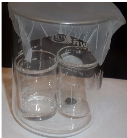
Figure 11: The anode (in the small beaker right) is chemically reduced under hydrazine vapor by sealing the anode in a large beaker with an open container (small beaker left) of liquid hydrazine monohydrate
