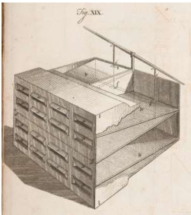
Figure 6: One of Stephen Hales' "ventilators" as described in his 1743 Description of Ventilators . Image credit: Wellcome Collection. Attribution 4.0 International (CC BY 4.0)
