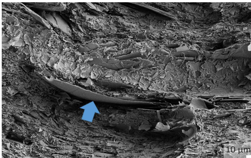
Figure 28 SEM image of 35% G-PEEK - Cycle 3, Graphite shown by arrow.
