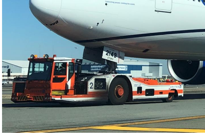
Figure 1 Pushback tractor or "Super tug" at Newark Liberty International Airport
