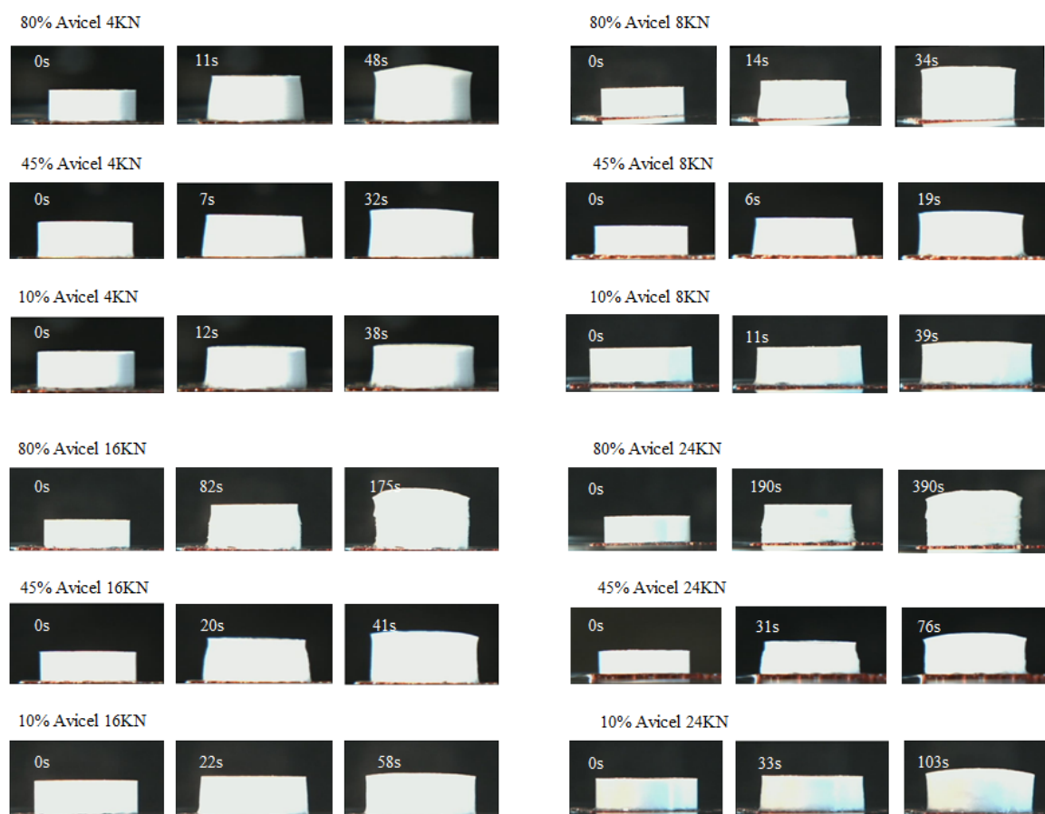
Figure 3.4 Swelling Processes of 80% Avicel, 45% Avicel, 10% Avicel and 4KN, 8KN, 16KN, 24KN.
