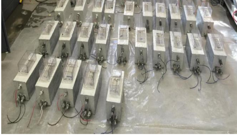
Figure 1 Samples of Corrosion Tests
