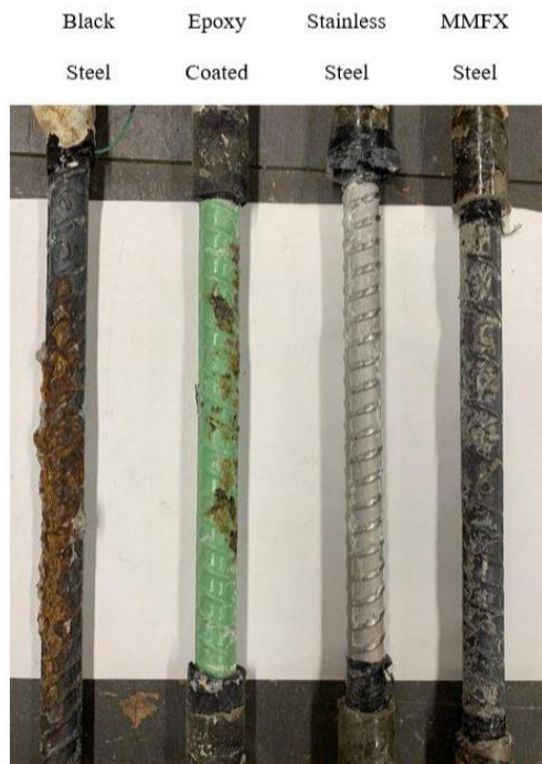
Figure 8 Different Types of Corroded Rebar
