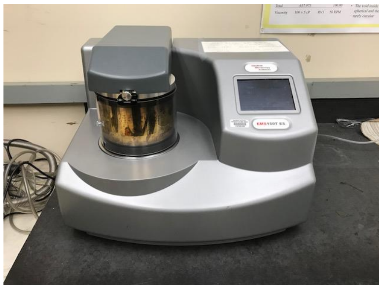
Figure 3-9 EMS150T E5 Sample Coater
