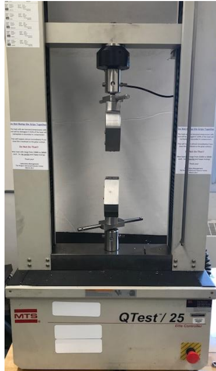
Figure 3-20 MTS QTest / 25 Tensile Testing Machine
