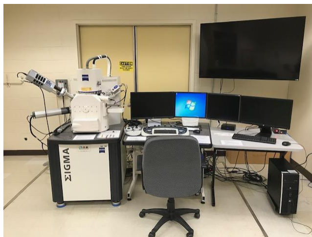
Figure 3-10 Sigma Field Emission Scanning Electron Microscope with Oxford EDS
