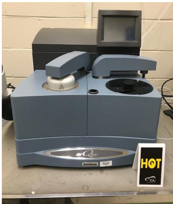
Figure 3-22 TA Instruments Q1000 Differential Scanning Calorimeter
