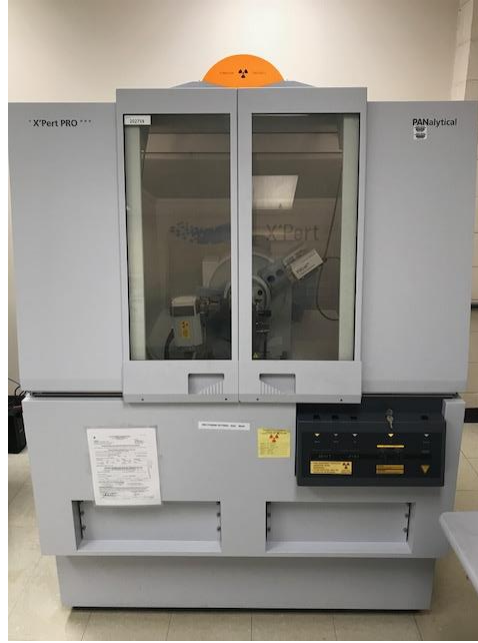
Figure 3-16 Philips XPERT Powder X-ray Diffractometer
