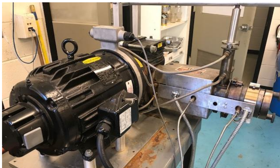
Figure 3-6 High Shear Batch Mixer
