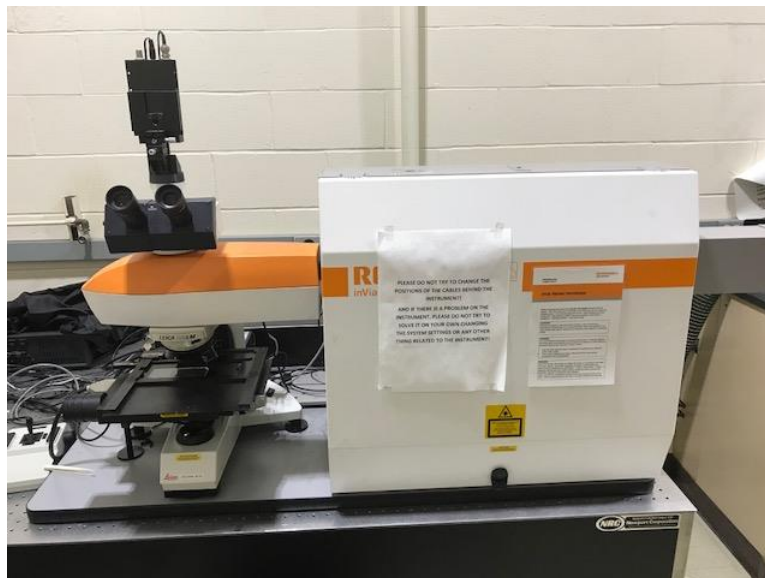
Figure 3-19 Renishaw Raman Spectrometer
