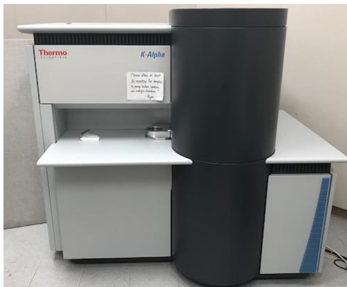
Figure 3-14 Thermo Fisher Scientific X-ray Photoelectron Spectrometer
