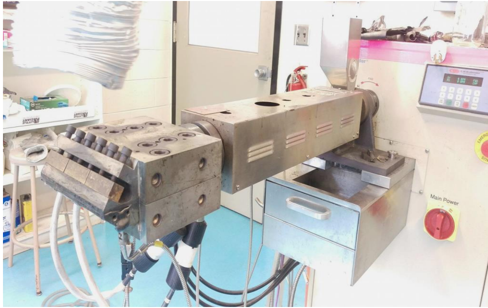
Figure 3-7 Brabender Intelli-Torque Extruder
