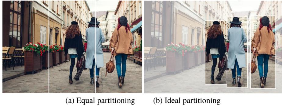
Fig. 4.1 Examples of video frame partitioning. The simple partitioning method in (a) may split pixels of the same object into multiple parts and yield poor inference results. We can achieve much better partitioning using ELF, close to the ideal partitioning shown in (b)
