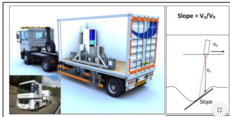
Figure 1 TSD equipment and operating method (Katicha et al., 2014)
