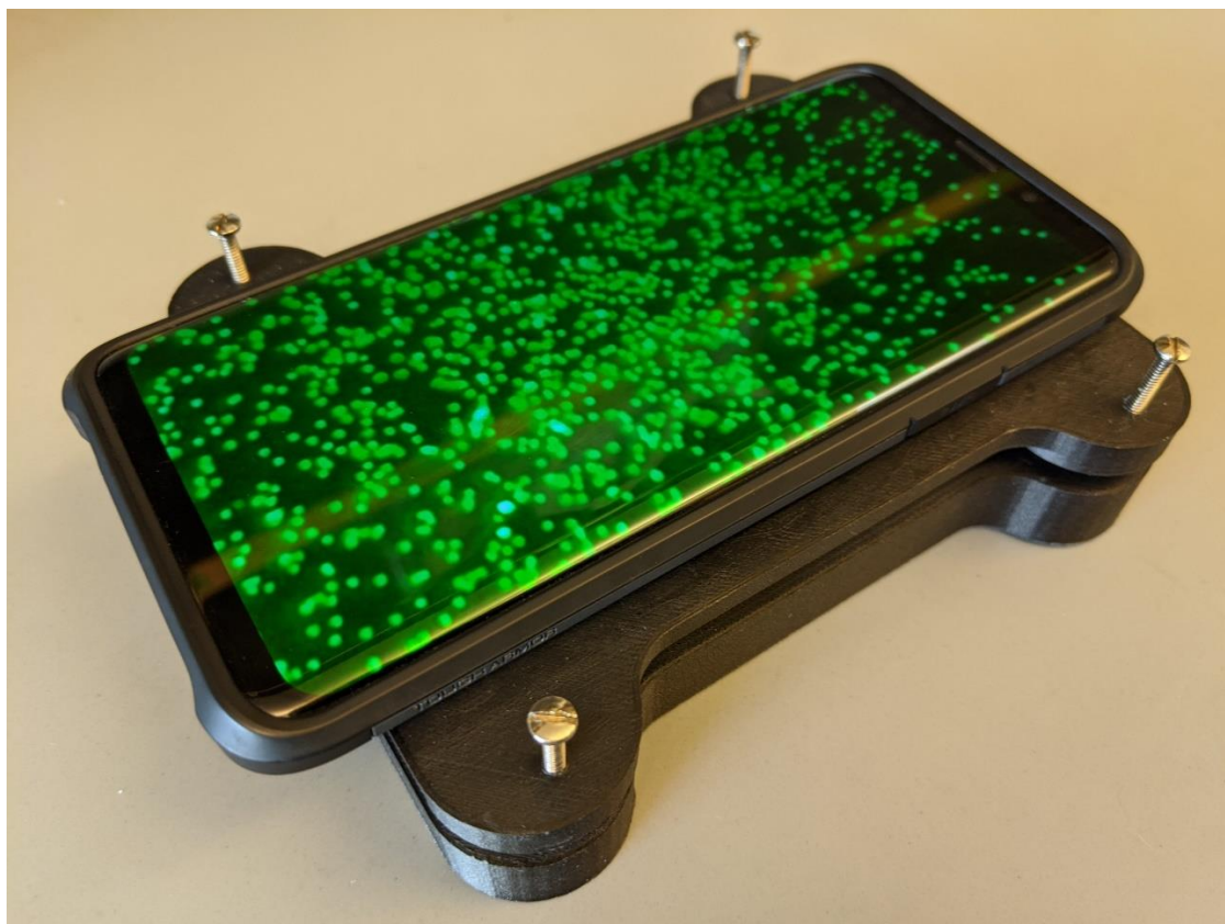
Figure 2-2 3D printed smartphone based fluorescent microscope working in conjunction with a Samsung Galaxy S9+. Reproduced from Ref. [26] with permission from the Royal Society of Chemistry.
