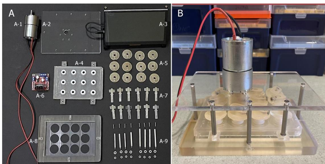
**Fig. 5 Spinfinity: a miniaturized bioreactor.** (A) 3D printed and hardware components of the bioreactor. (B) Fully assembled bioreactor.
