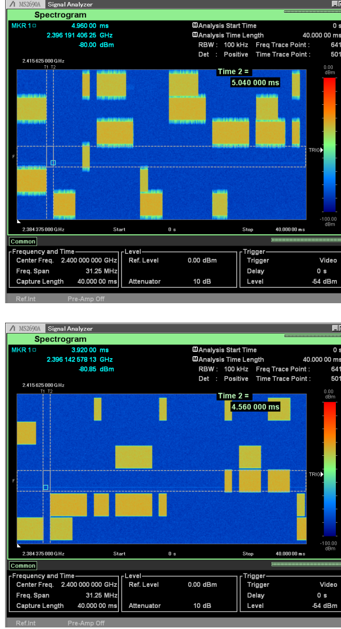
Figure (3.3) Comparison of McF-TDMA feature. (a) FPGA-based filters disabled. (b) 128 order FPGA-based FIR filter enabled results in significantly lower out-of-band transmissions and thus reduced interference in adjacent bands.
