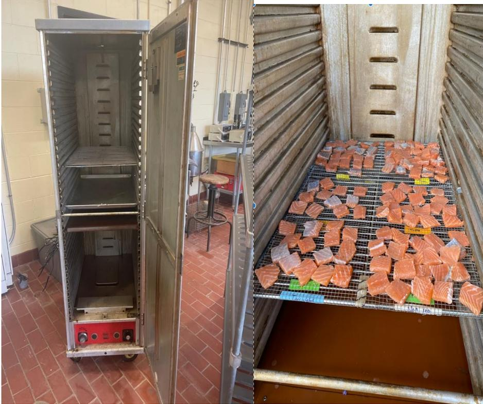
**Fig 4.2.** (a) The cold smoker used in this study (b) Set up of the cold smoking experiment.
